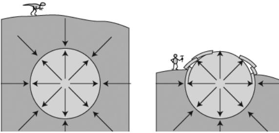
Outcrop boulders tend to form thin slabs, caused by a process called exfoliation. As the granite pluton cooled deep within the earth, outward pressure balanced inward pressure. However, as erosion removed the overlying rock, pressures were no longer balanced. The rock expanded and formed horizontal cracks. Look for vertical drill holes from quarrying in the past.
